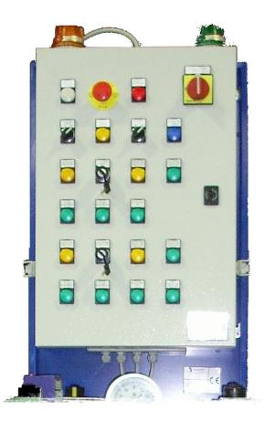
The electrical control panels are specifically designed to supply power to the several instrumentation and equipment installed in the filling station and control them all. Main control panels are designed to start and stop the pumps, open and close the valves, detect temperatures and pressure by electronic sensors installed on field. They are available with electro-mechanic logic control or with PLC and relevant software logic control of the pumping and filling process.
