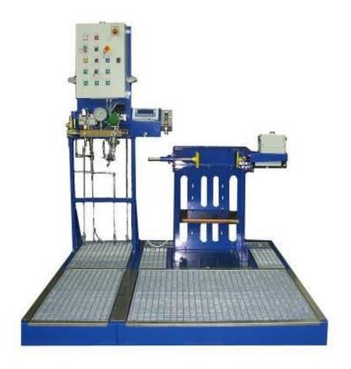
Complete installation for CO<sub>2</sub> cylinders filling with one filling outlet
