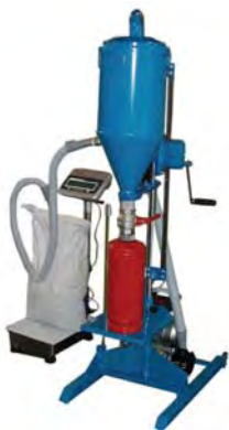
FILLING OF PORTABLE EXTINGUISHER
