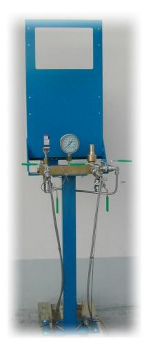
Manually controlled, the FCD22 unit allows to fill cylinders and extinguishers with CO2 transferred from a cryogenic tank. The operator acts on the check valves manually according to the information supplied by the control weighing scale displays. Bundle filling can optionally be obtained on a third weighing appropriate scale
