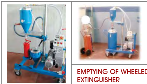
FILLING OF PORTABLE EXTINGUISHER
